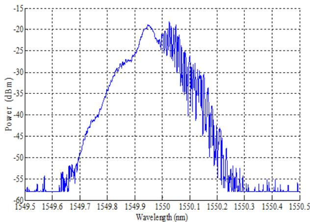
**Figure 3.** OSA displays the output of the system shown in Figure 2 (Laser Power 20 mW, Fiber loop mirror length 6.6 Km and OSA Resolution 0.07 nm)
