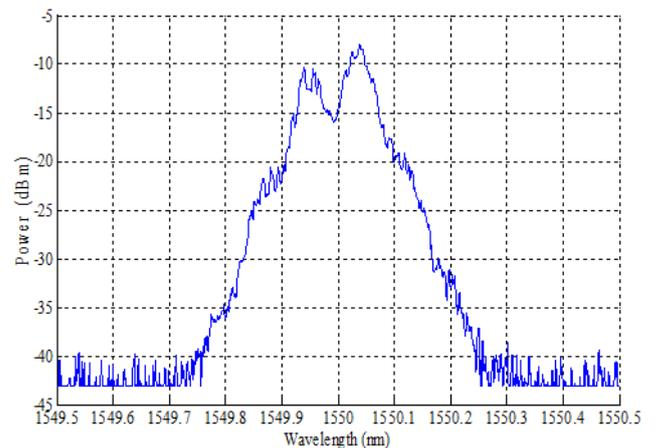
**Figure 5.** OSA displays the output of the system shown in Figure 4 (Laser Power 15mW, Fiber loop mirror length 6.6 Km and OSA Resolution 0.07 nm)
