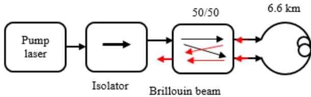
**Figure 2.** Brillouin beam generation using fiber loop mirror.
