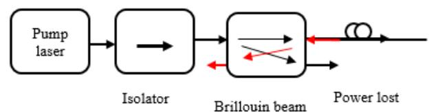
Figure 1. Direct technique to generate Brillouin beam
