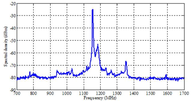
**Figure 7.** RF spectrum analyzer display (VBW =100 KHz and RBW=1 MHz)
