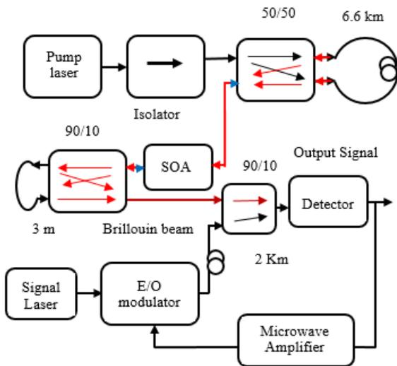
**Figure 6.** OEO using Brillouin beam generated by two fiber loop mirrors technique.
