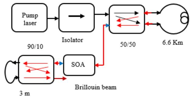
**Figure 4.** Brillouin beam generation using double fiber loop mirror.
