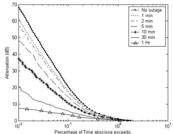
Figure 2: Rain attenuation exceedance for different outage tolerance configuration
