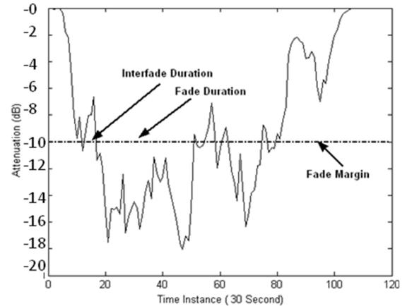
Figure 1: Typical rain attenuation occurring in India at 30 GHz.
