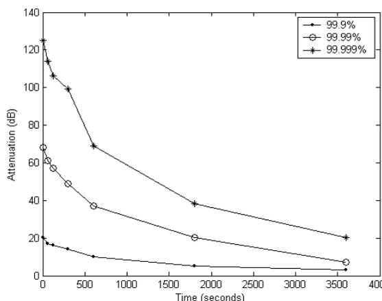
Figure 3: Variation of required fade margin with outage tolerance time for maintaining the minimum link availability
