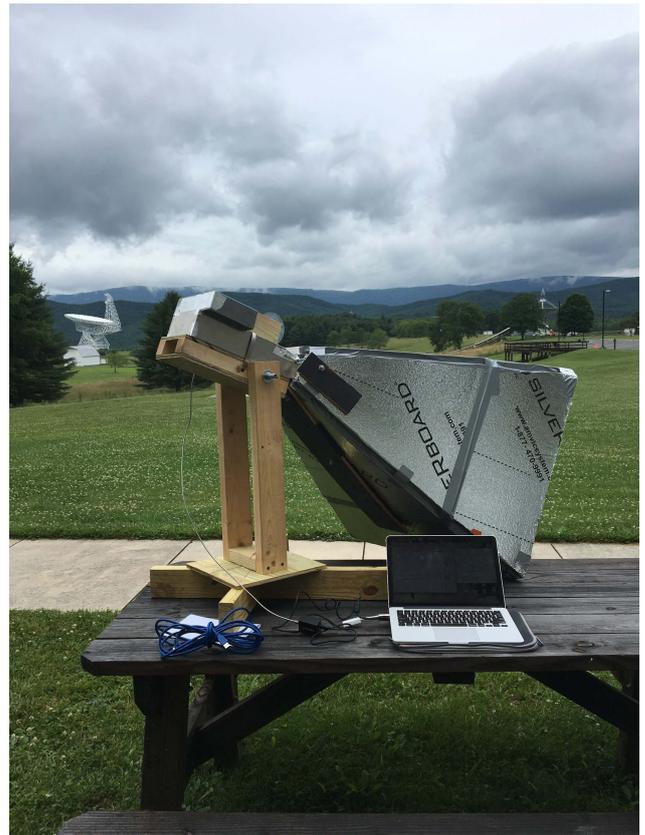
**Figure 1.** Neutral Hydrogen horn antenna taking a hot load measurement of the ground near the Green Bank Telescope.
