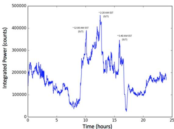
Figure 4. Spikes in intensity captured by the loop antenna in September 2017. These spikes correspond with ionospheric disturbances.
