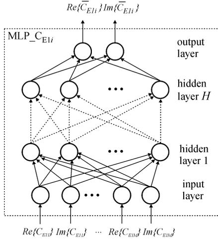
**Figure 3.** MLP architecture used in MLP\_C<sub>1m</sub> and MLP\_DoA networks
