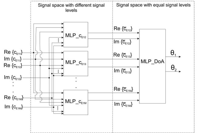
**Figure 2.** Architecture of the two-stage cascade neural model ( $\text{MLP\_C}$ )
