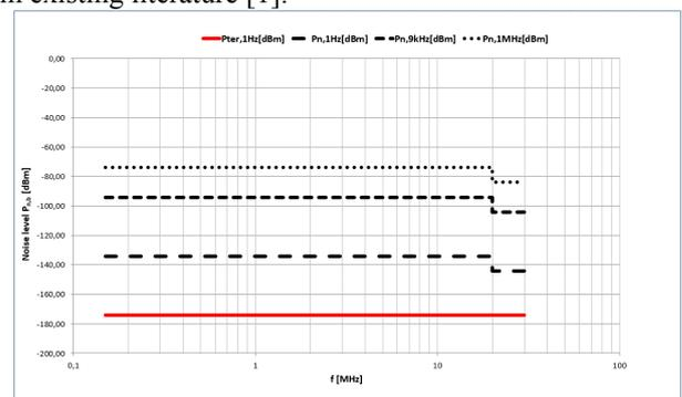
**Figure 1. Example values of thermal noise levels  $P_{ter,b}$  and conducted background noise levels  $P_{n,b}$  for a frequency range of 150 kHz – 30 MHz, as presented in existing literature [1]**
