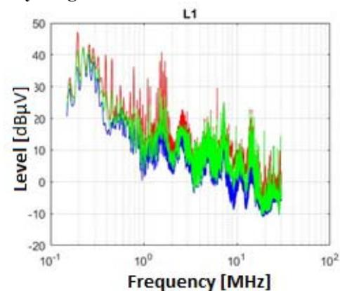
**Figure 6. Maximum (red), minimum (blue) and average (green) values for the conducted background noise level  $U_{n,b}$  measured in the 150 kHz – 30 MHz frequency range on each low voltage power line  $L_1$**
