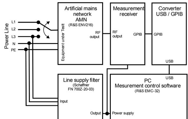
**Figure 3. Block diagram of a measurement system designed to measure conducted thermal noise voltage levels  $U_{ter,b}$  and conducted background noise  $U_{n,b}$  for a frequency range of 150 kHz – 30 MHz**
