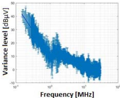
**Figure 8. Distribution of values measured in the frequency range from 150 kHz to 30 MHz on all low voltage power supply lines:  $L_1$ ,  $L_2$ ,  $L_3$  and  $N$**
