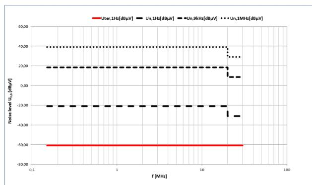
**Figure 2. Mean root values of thermal noise voltage levels  $U_{ter,b}$  and conducted background noise  $U_{n,b}$  for a frequency range of 150 kHz – 30 MHz**
