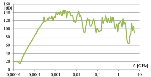
**Figure 5. FN 700Z-20-03 filter attenuation in the frequency range of 150 kHz – 30 MHz**
