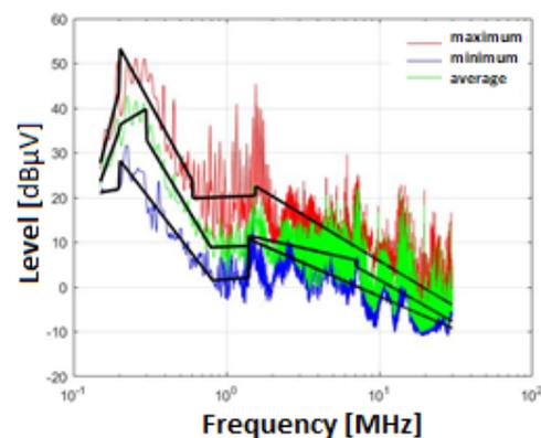
**Figure 7. Maximum (red), minimum (blue) and average (green) values along with approximation functions for the conducted background noise level  $U_{n,b}$  measured in the 150 kHz – 30 MHz frequency range on all low voltage power lines:  $L_1, L_2, L_3$  and  $N$**
