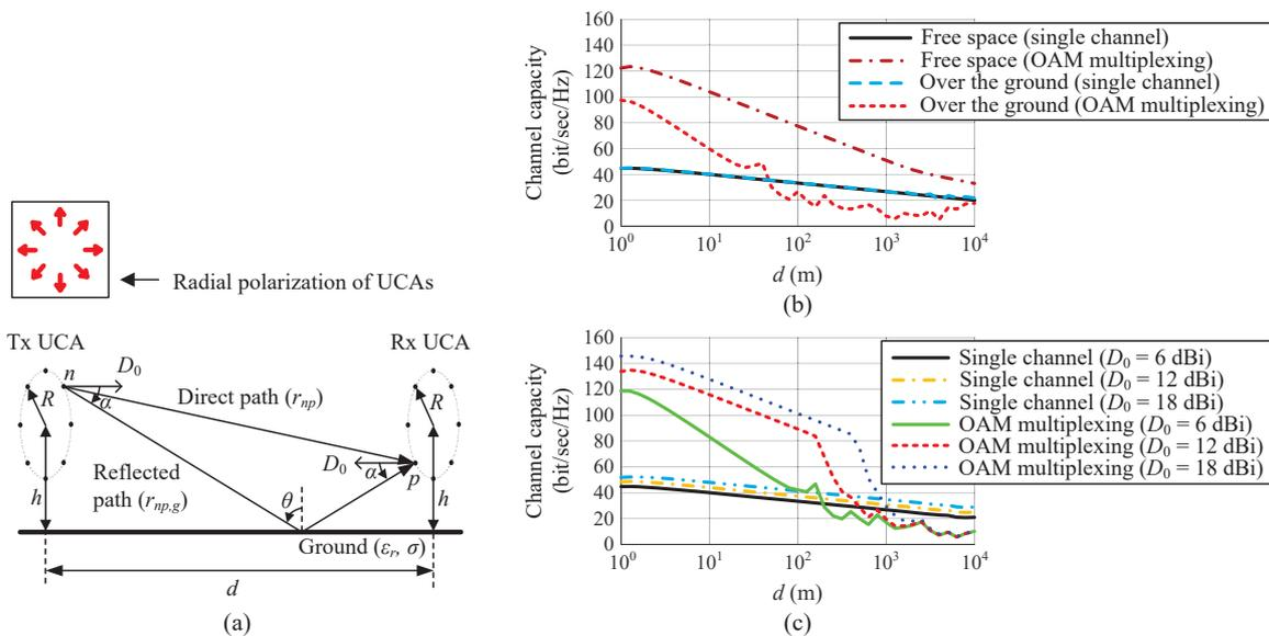
**Figure 1.** OAM system with radial UCAs. (a) OAM transmission link over the flat ground. (b) Channel capacities of an OAM multiplexing channel and a single channel in free space and over the ground. (c) Channel capacity vs. the directivity of UCA elements over the ground.
