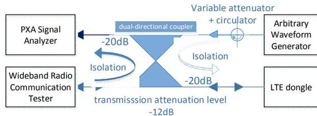
**Figure 1.** Schematic diagram for a LTE communication in the presence of EM interferences.
