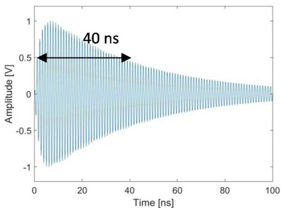
**Figure 3.** Representation of the EM interference signal model in time domain.
