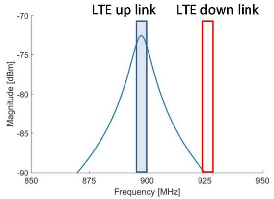
**Figure 4.** Representation of the EM interference signal model in frequency domain.
