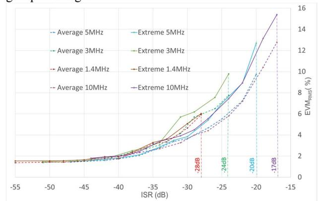
**Figure 5.** EVM as a function of the ISR, for a QPSK modulation.
