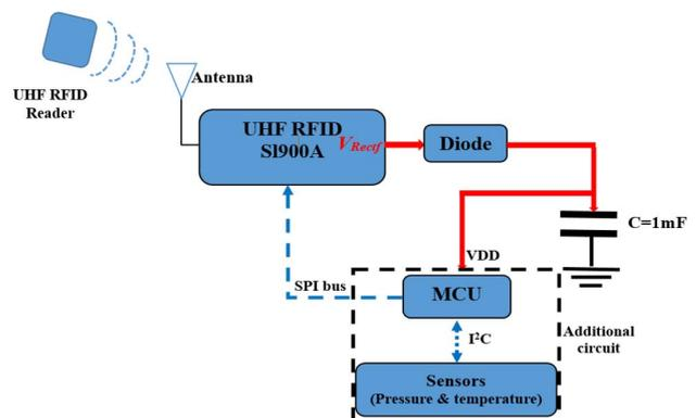
Figure 1. The block diagram of the proposed tag architecture
