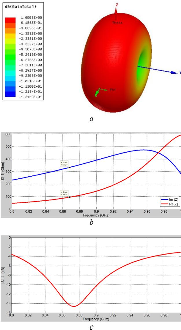
**Figure 3.** Antenna simulation results (a) Radiation pattern at 868 MHz ( $\phi = 90^\circ$ ), (b) input impedance, (c) return loss
