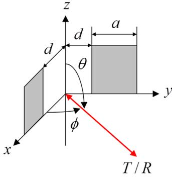
**Figure 1.** Configuration 1: two PEC square plates at  $90^\circ$  to each other.
