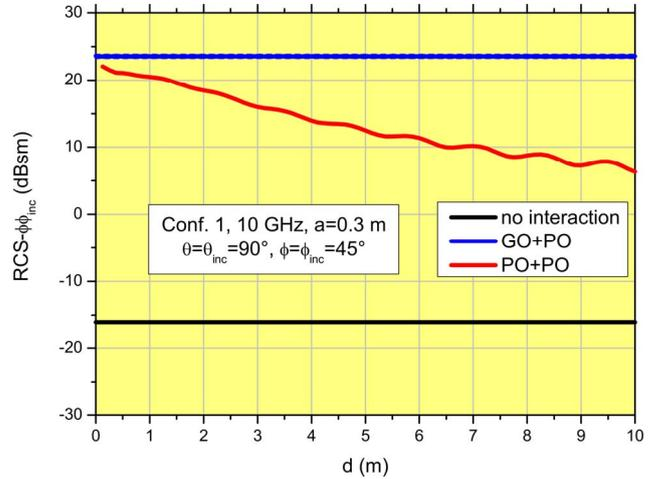
**Figure 3.** Backscattering cross section of configuration 1 as a function of the distance between the plates, with interaction between the plates neglected (black) or included and calculated by either GO (blue) or PO (red). The electric field vector is in the  $x$ - $y$  plane.
