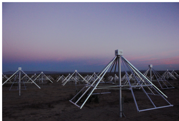
Figure 1. LWA-SV radio telescope: An photo taken from the middle of the array showing several of the dual-polarization dipoles.
