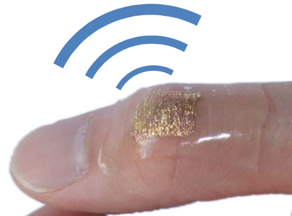
Figure 1 Vision of bendable & stretchable radio band-aid
