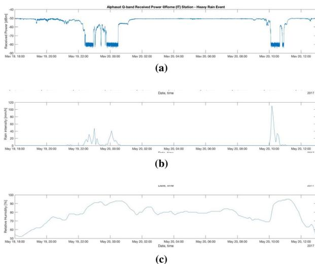
**Figure 4.** Rain event acquired by the Q-band receiver with tracking system (4a) and the in-site meteorological station (4b,4c).
