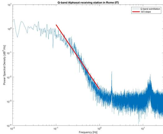
**Figure 6.** Q-band receiver scintillation Power Spectral Density in clear air condition.
