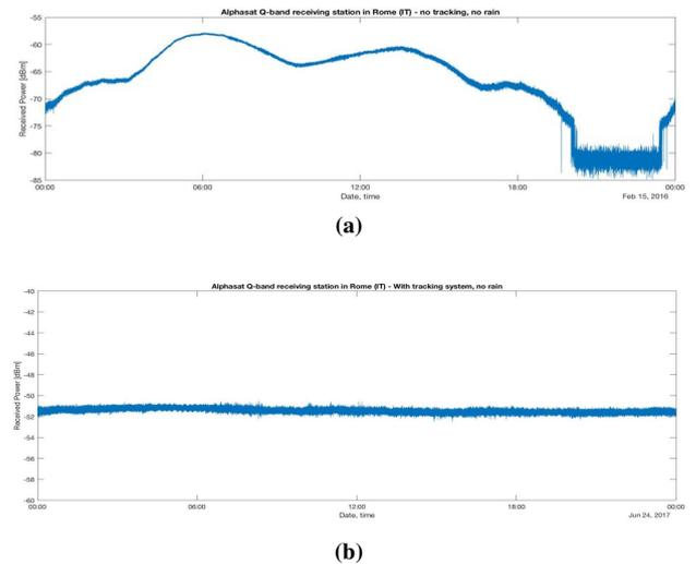
**Figure 3.** Data acquisition before and after the tracking system installation.
