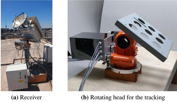
**Figure 1.** Alphasat Q-band receiving station in Rome
