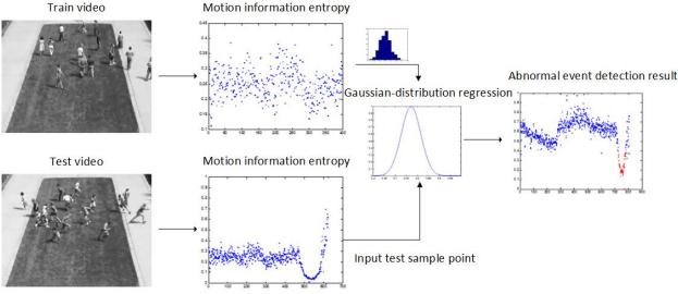
**Figure 1.** Overview of proposed global abnormal event detection based on motion information entropy.
