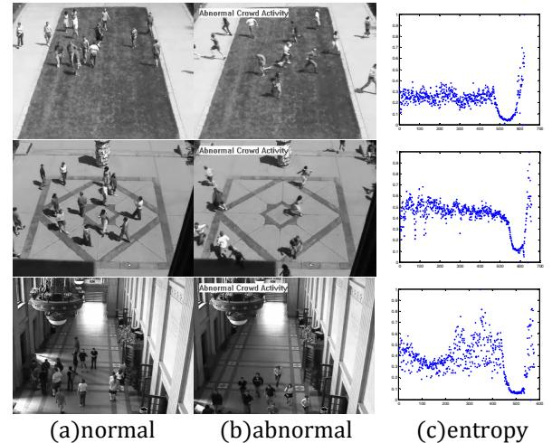
**Figure 2.** Motion information entropy distribution in different scenes (a) normal behavior, (b) abnormal behavior, (c) the distribution of motion information entropy
