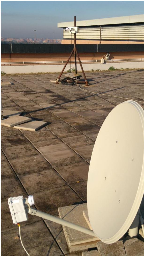
Figure 2. Smart LNB and collocated laser disdrometer at CNR-ISAC in Rome
