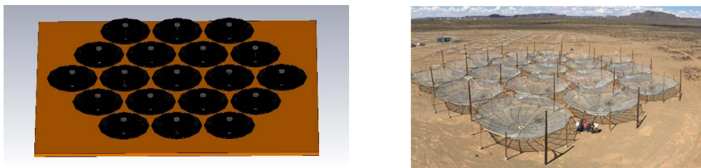
Figure 1. CST electromagnetic simulation and picture of the first 19 elements built in the Karoo desert
