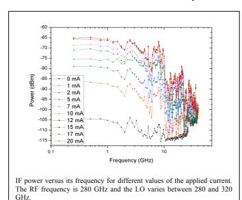
Unipolar nanodiodes have been used as mixers for heterodyne detection of two THz incoming radiations at room temperature; the resulting signal has been transposed into a measurable GHz IF-signal. In this first implementation, the IF signal has been tuned between 0 GHz and 40 GHz with a dynamic range of 70 dB combining the advantages of a large IF-bandwith simultaneously with reasonable conversion losses.
