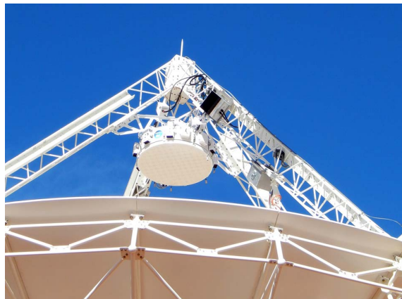
Fig. 1. The first Mk II PAF on ASKAP antenna 29 at the Murchison Radio-astronomy Observatory.
