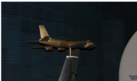
Figure 1: Scale model of Boeing in the Compact Range.
