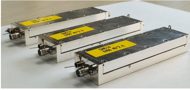
Figure 2. LNA chassis: 82×28×15 mm for LNA1 and 98×28×15 mm for LNA2 (excluding connectors).
