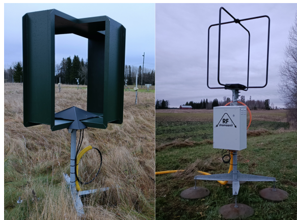
Figure 1. The transmitter (left) and receiver (right) antennas of the FMI's ionosonde in Southern Finland.
