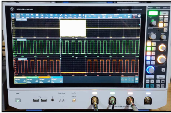
Figure 7. HPM-induced logic error from Logic Hold.
