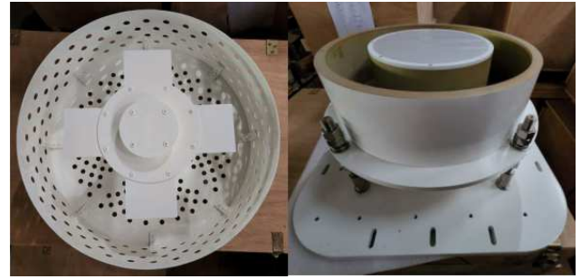
Figure 2. Left: The cavity dipole feed for 327MHz and 654MHz. Right: The longitudinal slot horn feed for 1400MHz.
