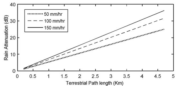
**Figure. 4** Plotting of rain attenuation as a function of terrestrial path length for different rain rates 50, 100 and 150 mm/hr.
