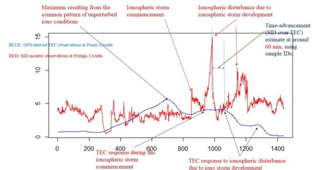
**Figure 4.** Observed consistent time/phase advancement of SID time series over the TEC ones
