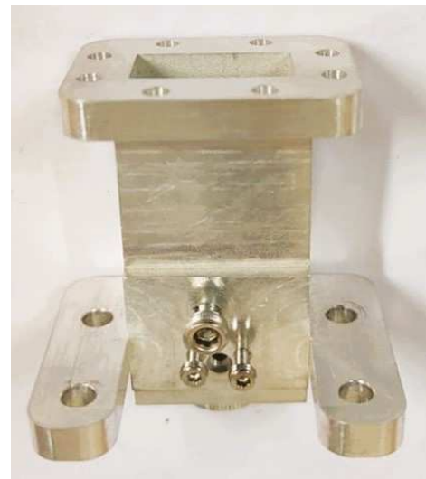
Figure 10. The fabricated H plane waveguide with tuner
