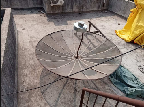
Figure 3 The setup consisting of the dish the feedhorn and the LNA balanced on bricks. A RG-58 coaxial cable runs from the feed to the RTLSDR indoors.
