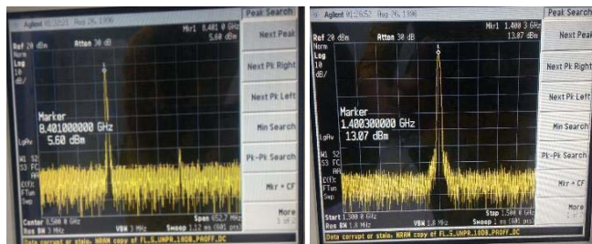
Figure 8: Testing results of Local oscillator chain 1 and 2
