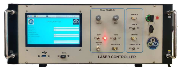
Figure 3. An in-house developed complete laser controller unit for current, temperature and piezo control of ECDL laser.
