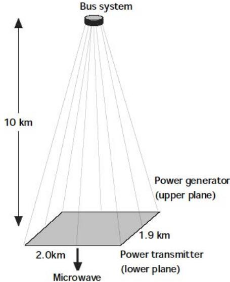
Fig. 2.4.11 1GW class Tethered-SPS
