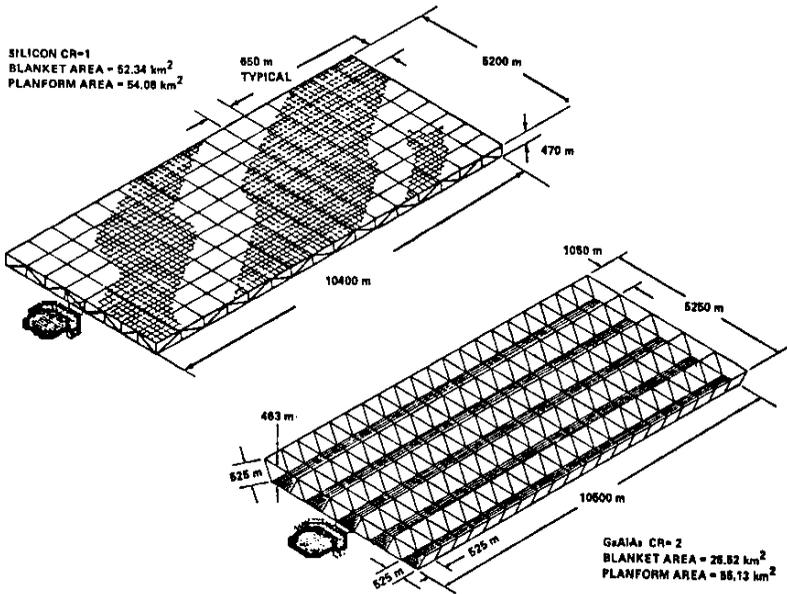
Fig. 2.4.2 NASA-DOE SPS Reference Model
