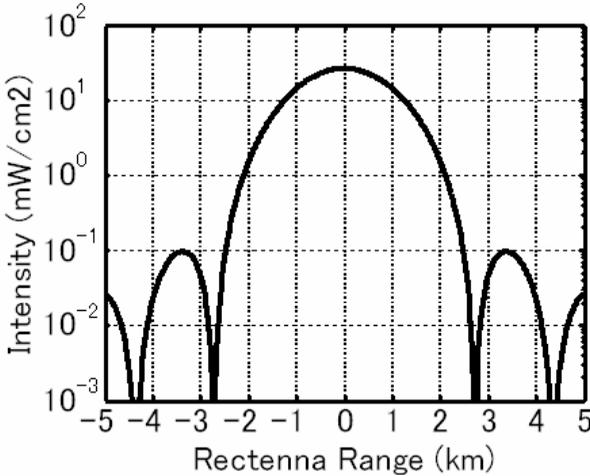
Fig. 2.2.1 Typical power density at a rectenna site
