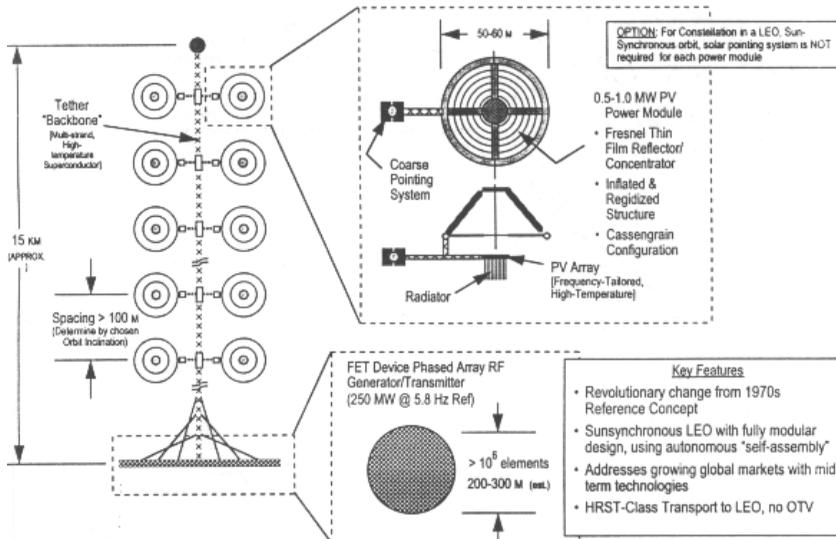
Fig. 2.4.4 The "Sun Tower" SSP Concept (MEO constellation)
