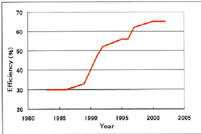
Fig.2.3.12 Trend of Efficiency of TWTA<sup>45</sup>
