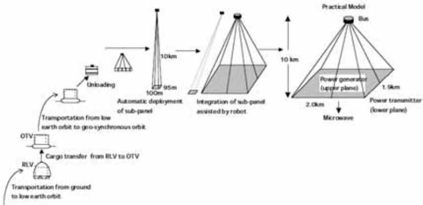
Fig. 2.4.13 Overall construction scenario
