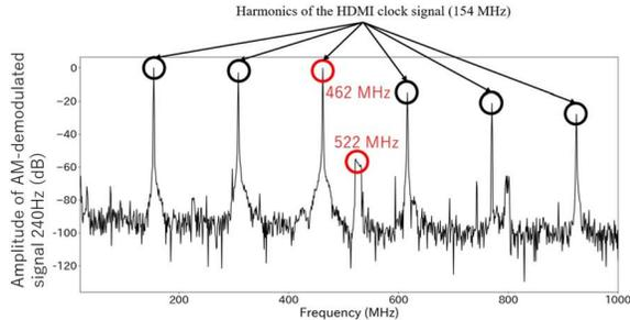
(a) Amplitude of AM-demodulated signal 240Hz
