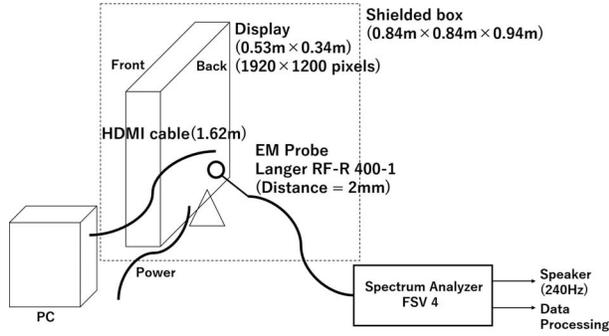
Figure 3. Experimental setup.
