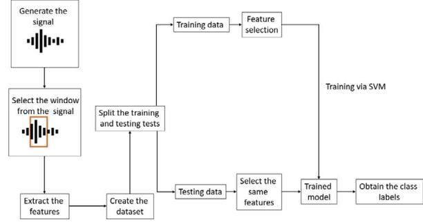
Figure 1. Interference detection process.
