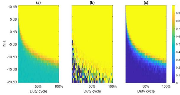
Figure 5. (a) Accuracy, (b) precision, and (c) recall of the pulse-blanking detection method as a function of INR and DC.
