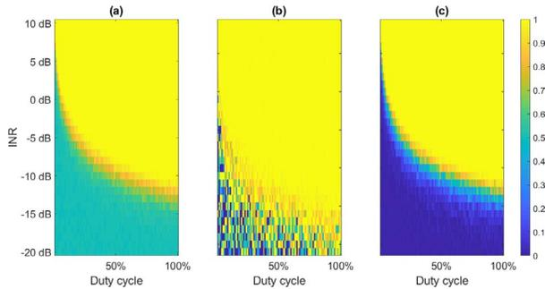
Figure 6. (a) Accuracy, (b) precision, and (c) recall of the OR method as a function of the INR and DC.
