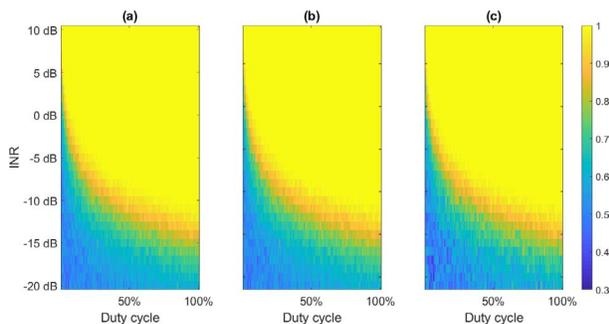
Figure 8. (a) Accuracy, (b) precision, and (c) recall of the proposed method that uses kurtosis and the received signal power as features as a function of the INR and DC.
