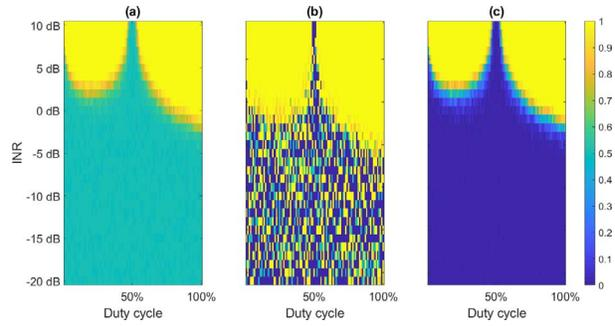
Figure 4. (a) Accuracy, (b) precision, and (c) recall of the kurtosis-detection method as a function of the INR and DC.
