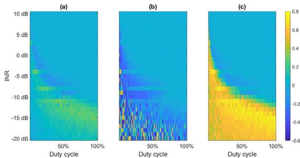
Figure 7. (a) Accuracy, (b) precision, and (c) recall difference between the proposed RFI detection method and the OR method as a function of the INR and DC.
