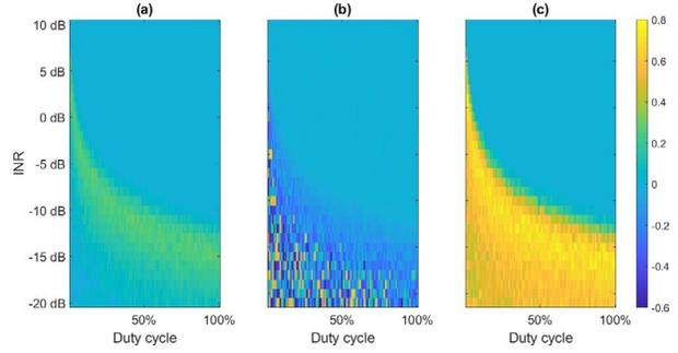
Figure 9. (a) Accuracy, (b) precision, and (c) recall difference between modified classifier and the OR method as a function of the INR and DC.
