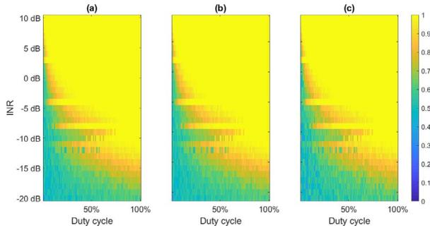
Figure 2. (a) Accuracy, (b) precision, and (c) recall of the proposed RFI detection method as a function of the INR and DC.
