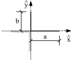
Figure 6. Right-angle wedge with two metal baffles.
