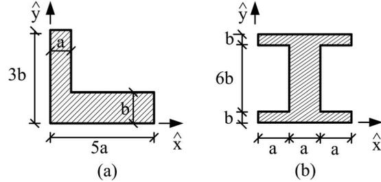
Figure 9. (a) L and (b) I beams.
