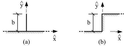
Figure 4. (a) Strip and (b) step on a metal plane.
