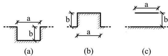
Figure 5. (a) Rectangular trench, (b) rectangular ridge, and (c) strip on a metal plane.
