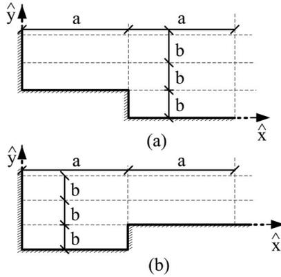
Figure 2. (a) Step and (b) trench in a dihedral reflector.
