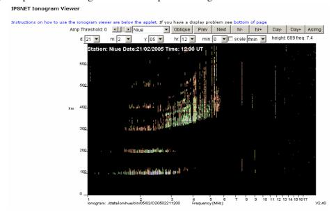
The next example is a night-time ionogram showing equatorial spread F. Past observations from both Raratonga and Maui suggest equatorial spread F will be observed at Niue.
