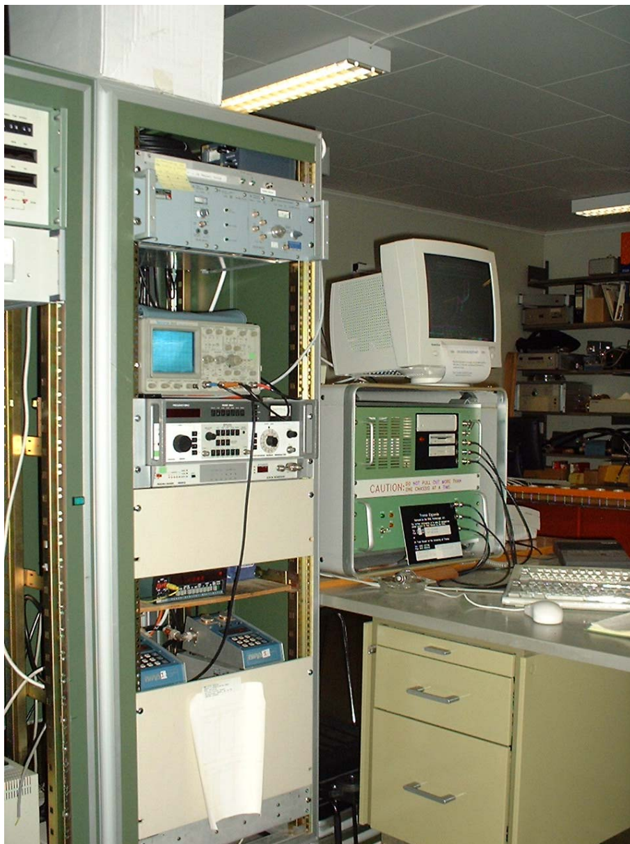
Fig. 7. The Lowell ionosonde. The Lowell unit itself is beneath the computer monitor. The rack to the left contains frequency reference equipment including synchronisation with nearby instruments. (Photo: Bjørnar Hansen)
