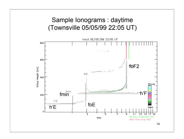
(Note that h'F is marked too low, and foE is too low. It is a result of how the plotting system works)
