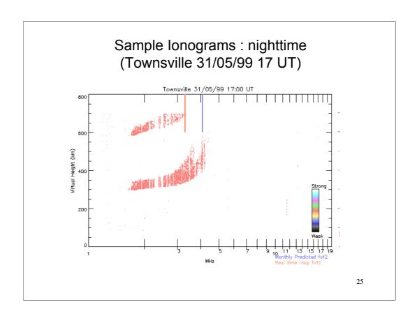
Now the spreading is more extensive, and scaling is harder. Extrapolation is more difficult, and the multiples give little guidance as they also are spread as well as being cut off by the display.
