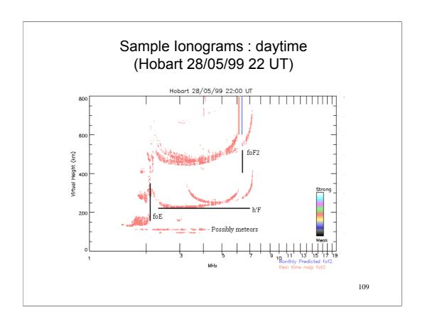
Meteors can be seen on most ionosondes. However, it depends on the time it takes to make an ionogram and the system sensitivity.
