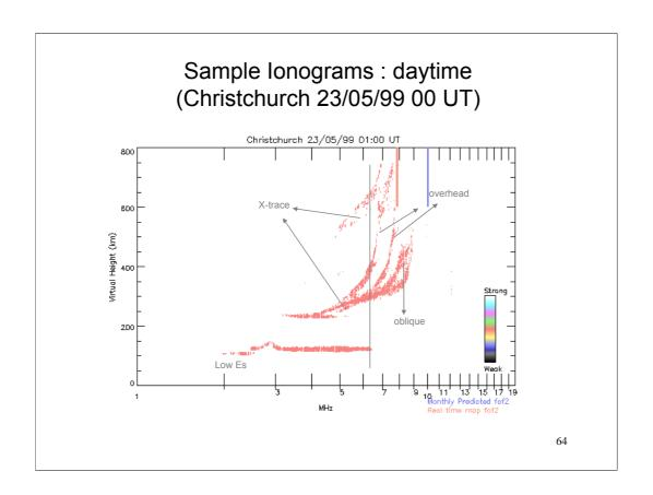
Note that there are two Es layers, a low layer from which fmin is scaled and a high layer. The difficult bit is to decide where foEs is.
