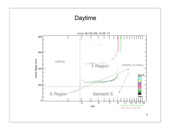
In daytime, the vertical dividing line runs through foE, the peak electron density of the E region.
