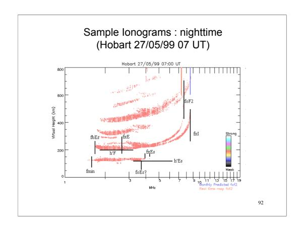
The important point here is to recognise that x-trace F region extends below the top of the Es layer. So both traces are present in the Es layer.
