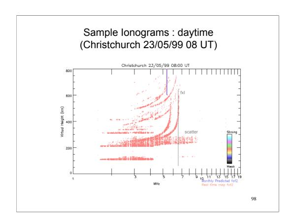
Clearly there is ground scatter present and it should be ignored in scaling fxI and the Es parameters. Why? Because it is due to a gradient and is therefore not an overhead return.
