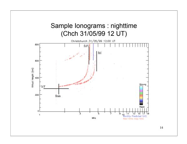
The base height of the F region, h'F, and the peak of the layer, foF2, define the layer reasonably well. For completeness, we should also add some information about the layer thickness. For the F region, this comes from scaling M(3000)F2, which can then be interpreted as the peak height of the F region.
