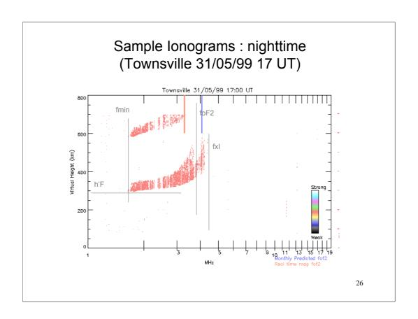
The issue of a weak trace near fxI is clearer on this example. Picking fxI is difficult to place with confidence, partly because some of the final returns would not be seen on a less sensitive display. It is a matter of judgment whether you seek to get information like this from an ionogram. The main thing is to be consistent in how you interpret such examples, both with your latter efforts, and those of others also scaling with you.
