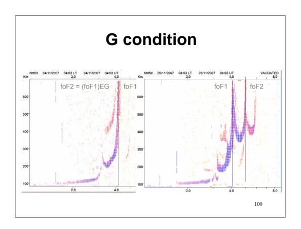
The correct scaling for foF2 is shown in both cases: when foF2 is not visible (the G condition) and when it is visible.
