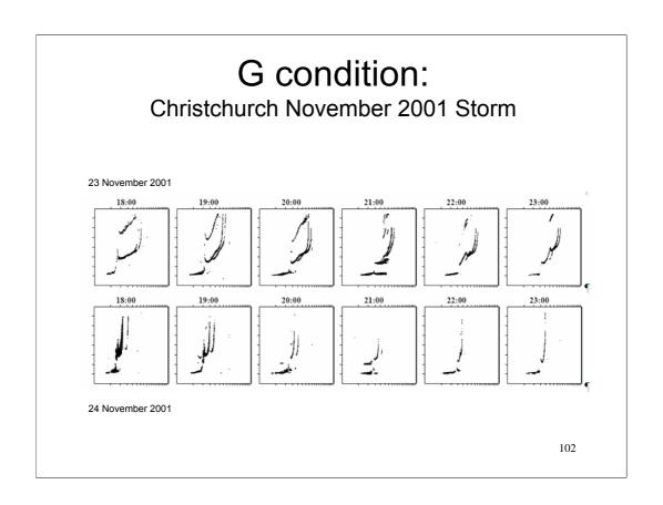
Here a sequence in time is shown for two successive days. The F1 region is poorly defined, but there is still a clear difference between the two days. On the 21<sup>st</sup> the storm has depressed F2 ionisation significantly.
