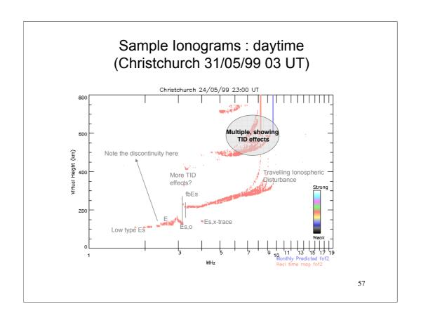
There is a low type Es layer here. It is apparent because of the change in altitude and discontinuity in the E region trace. Since fmin is controlled by the low layer, IPS would always scale L in the Es Type column, after the layer that contributed foEs.
