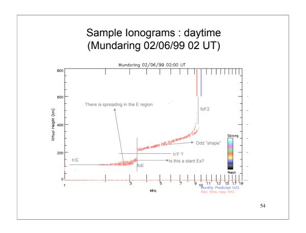
Spread Es is what is different here, and a possible slant Es trace also. This is a new condition and it may be worth noting its presence. IPS has special rules for noting this presence, although they do not reveal any special new knowledge.
