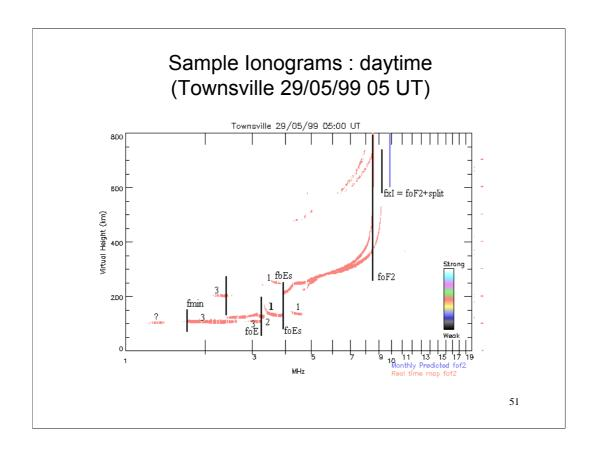
Fmin has been scaled from the clear continuous trace, ignoring the weak lower return. If this return appears on adjacent ionograms, then ignoring it is less realistic. A weak trace is usually thought to be weak both in signal strength, and in lifetime. This could be a low-type Es layer. If we believe it is definitely a return from the ionosphere, then fmin should be scaled off it. In IPS, we would be sure to note this is a low-Es layer by placing L in the type table.
