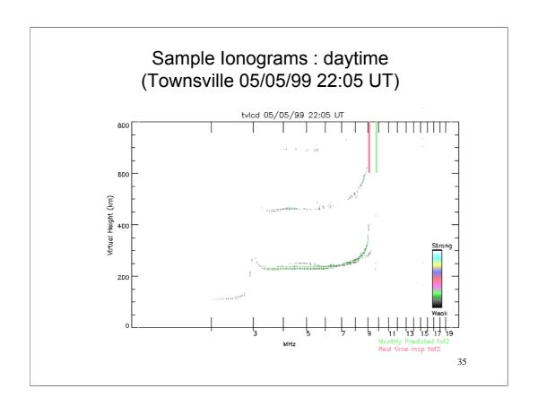
Daytime differs on two counts: more layers and absorption. These are a direct result of the presence of the sun. The sun's ionising radiation produces ionisation that can be observed using an ionosonde. As the incoming radiation changes, so the production of ionisation will respond, resulting in changes in the ionosphere.
