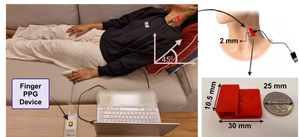
Figure 3. (left) Indicative data recording setup. The radar sensor is placed near the jugular vein for data collection, while PPG data are collected using the finger PPG device. The subject is reclined on a base with a sensor placed in reasonable proximity to the neck at an almost 45° angle to monitor cardiovascular parameters. (right) The 3D-printed plastic case is nearly the size of a 1-dollar Australian coin.
