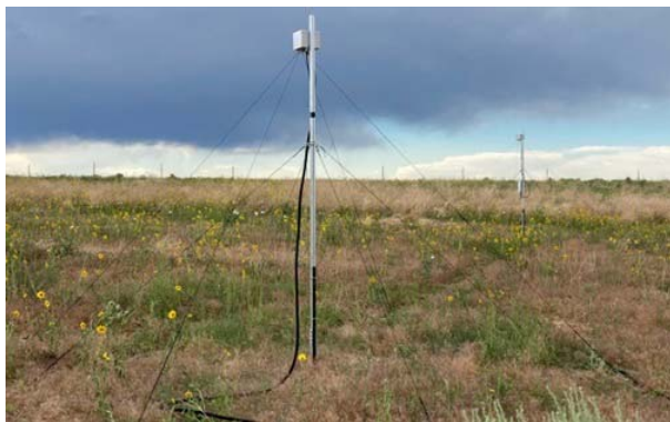
Figure 4. An inverted V dipole transmit antenna at the Platteville, Colorado, transmitter location.
