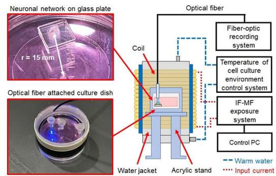
Figure 1. IF-MF exposure and nonconductive fiber-optic recording system with a hiPS cell-derived neuronal network cultured on a quartz glass plate. The culture dish and fiber optic are set in the IF-MF exposure coil for real-time detection of neuronal activity.
