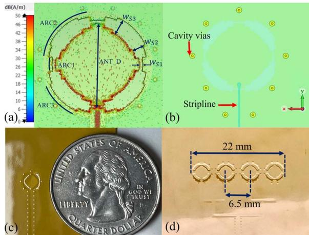
Figure 7. (a) The geometry and distribution of the current surface at the resonance frequency of the proposed antenna, (b) transparent top view, and (c) and (d) fabricated single and array antennas.
