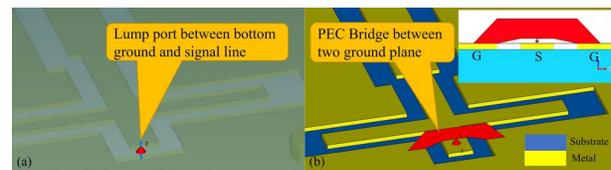
Figure 3. (a) Simulation setup for excitation of the Grounded Coplanar Waveguide (GCPW) line (method\_1) and (b) simulation setup for excitation of the GCPW line (method\_2).
