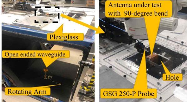
Figure 1. Far-field probe station setup.
