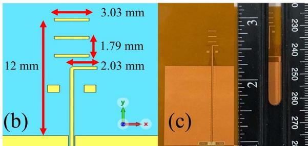
Figure 2. (a) The simulated  $S_{11}$  parameter of quasi-Yagi-Uda antenna for different scenarios. (b) Structure of the proposed antenna and (c) fabricated antenna in [20].
