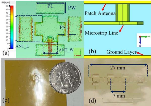
Figure 4. (a) The geometry and distribution of the current surface at the resonance frequency of the proposed antenna, (b) side view, and (c) and (d) fabricated single and array antennas.
