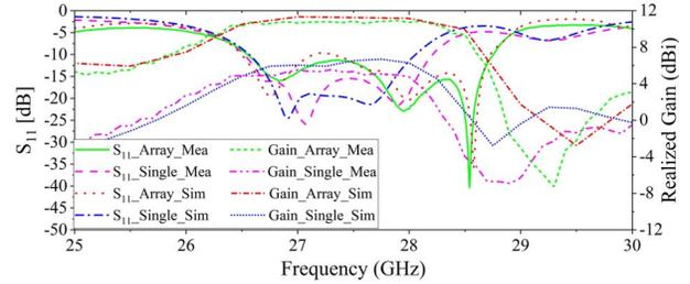
Figure 5. S parameter and realized gain of the proposed patch antenna versus frequency.
