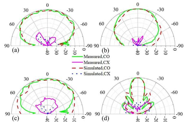
Figure 6. Simulated and measured radiation pattern of the proposed patch antenna at 28 GHz (a) E plane (single), (b) H plane (single), (c) E plane (array), and (d) H plane (array).
