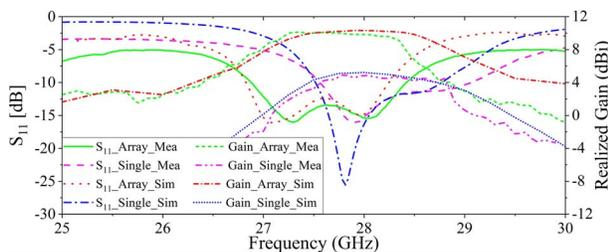
Figure 8.  $S_{11}$  parameter and realized gain of the proposed cavity slot antenna.
