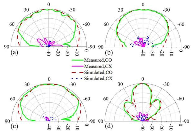
Figure 9. Simulated and measured radiation patterns of the proposed cavity slot antenna at 28 GHz (a) E plane (single), (b) H plane (single), (c) E plane (array), and (d) H plane (array).
