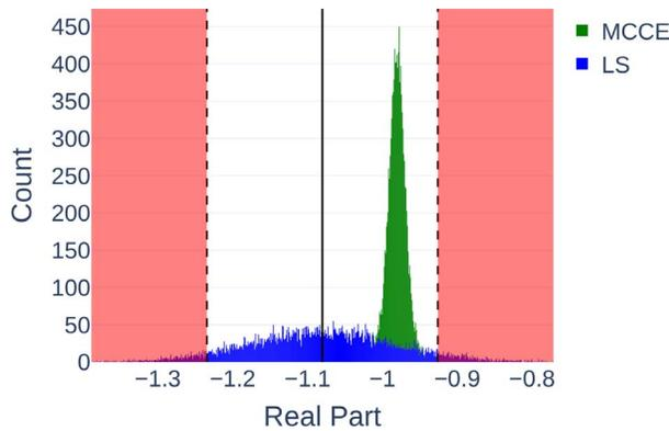
Figure 4. Example distributions of corrected values with a 64-QAM modulation. The real part of the value is shown centered around a single constellation point. Threshold boundaries are shaded in red, denoting areas of incorrect demodulation.
