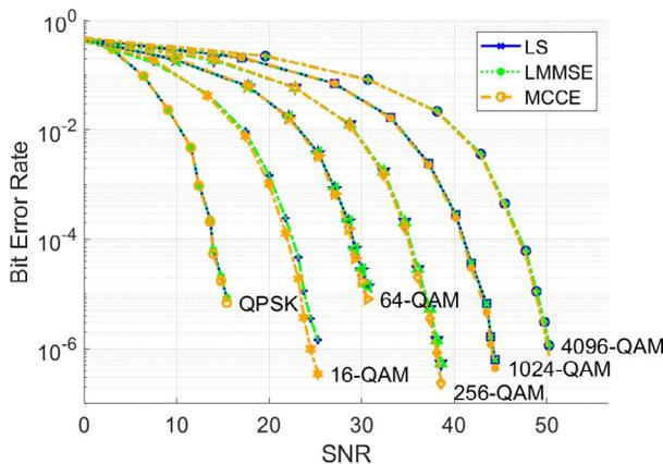
Figure 2. BER versus SNR for varying modulation schemes using the MCCE, LMMSE, and LS channel estimation techniques.
