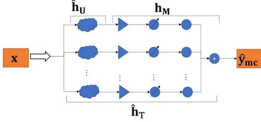
Figure 1. A depiction of the MCCE parameters. The input is given as  $\mathbf{x}$ , the MCCE output is  $\hat{\mathbf{y}}_{mc}$ ,  $\mathbf{h}_M$  is the modeled response,  $\hat{\mathbf{h}}_U$  is the unmodeled response, and  $\mathbf{h}_T$  is the total response.
