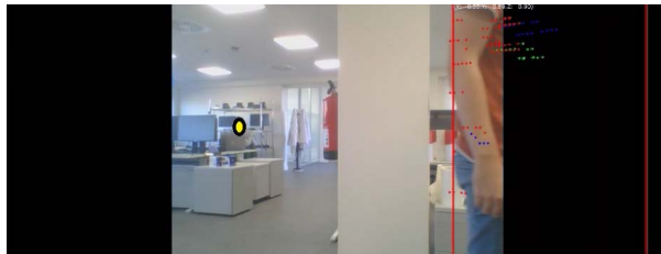
Figure 6. Enhancing the camera FoV with detection outside the camera FoV.
