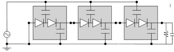
Figure 1. "Circuit diagram of single-ended three-stage VM."
