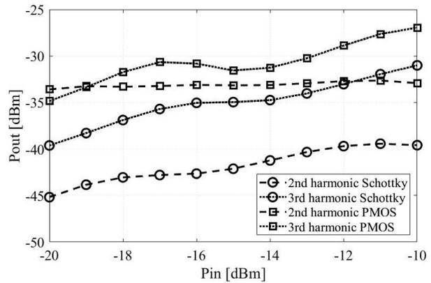
Figure 4. Harmonics generated with different input powers with a MN matched with  $-20$  dBm of input power with a modified PMOS diode and Schottky diode.
