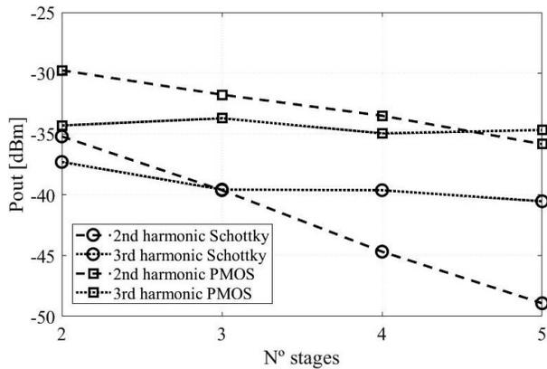
Figure 3. Harmonics generated with single-ended topology with PMOS and Schottky diodes.
