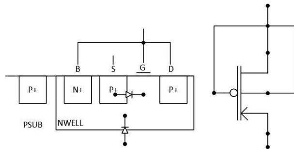
Figure 2. Diagram of the implemented modified PMOS diode.
