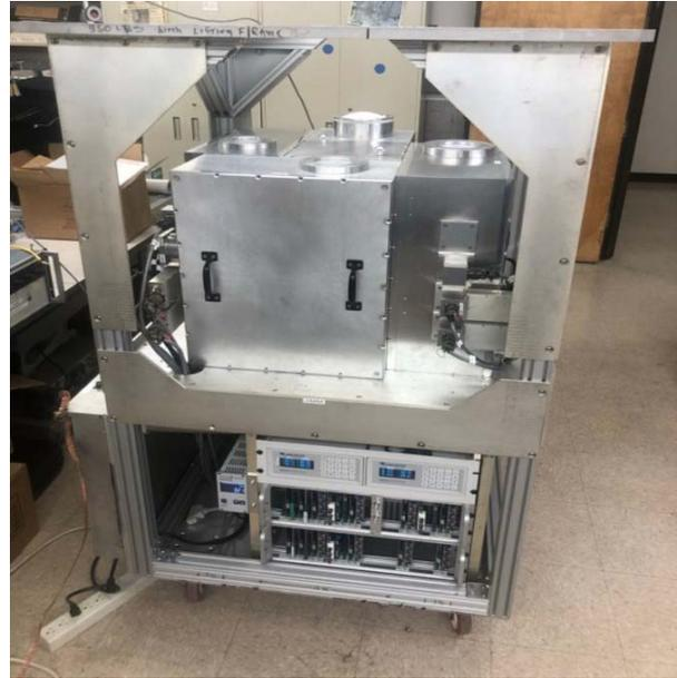
Figure 2. The complete receiver in its mounting frame. The dewar and its four modules are identified by their vacuum windows; the monitor and control electronics (temperature, vacuum, and bias control) are mounted under the dewar.
