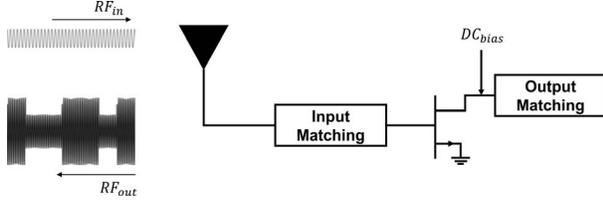
Figure 1. Block diagram of a reflection amplifier.
