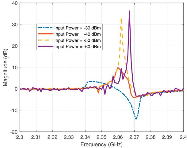
Figure 4. Power sweep analysis for 0.51 V case.
