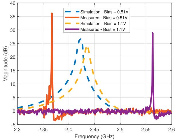
Figure 3. Simulated versus measured results with input power of  $-60$  dBm.
