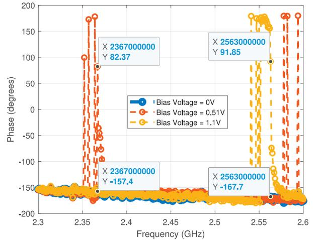
Figure 6. Phase comparison for the different bias points with input power of  $-60$  dBm.
