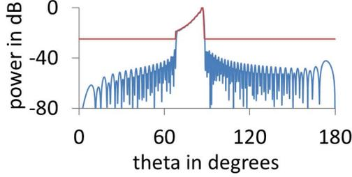
Figure 2. Synthesized uniform phase power pattern (blue) and mask (red).
