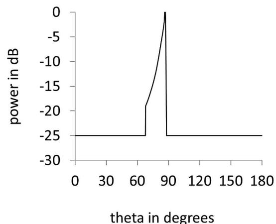
Figure 1. The desired far-field power pattern.
