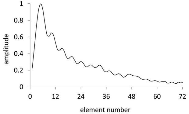
Figure 5. Optimum aperture amplitude distribution.
