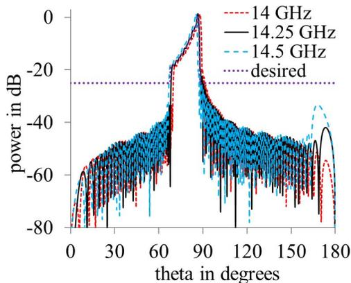
Figure 7. Optimized synthesis of the array power pattern.
