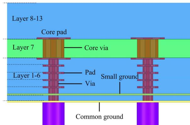
Figure 2. Stack up of the proposed DBDP element.
