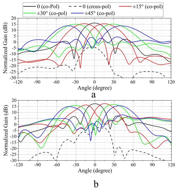
Figure 5. Simulated realized gain patterns in E plane for different scanning angles operating at (a) 28.5 GHz and (b) 38.5 GHz.
