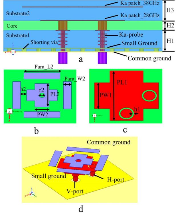
Figure 1. Layout of the proposed DBDP element. (a) Side view. (b) Top view of the higher band patch. (c) Top view of the lower band patch. (d) Perspective view of the lower band, higher band antenna, common, and small ground planes.
