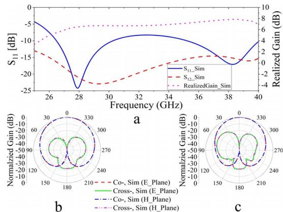
Figure 3. (a) S parameter and realized gain of the proposed single element. Normalized E\_plane and H\_plane radiation pattern at (b) 28.5 GHz and (c) 38.5 GHz.
