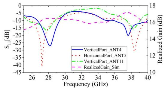
Figure 6. The active reflection coefficient for the  $45^\circ$  scanning angle (both polarization) and realized gain of the proposed antenna array.
