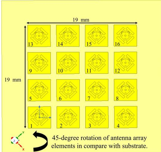
Figure 4. Configuration of the proposed antenna array.
