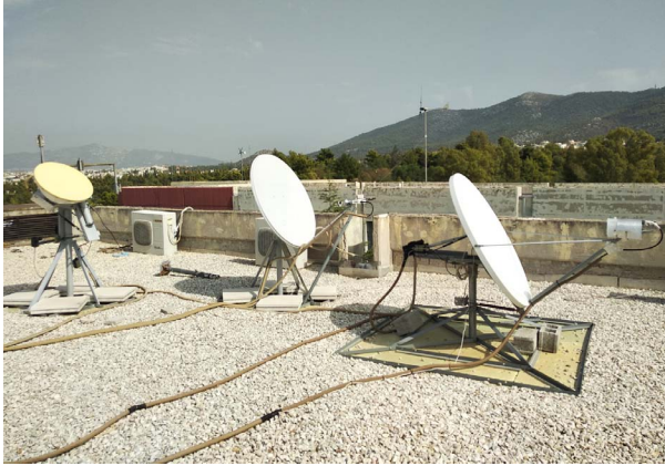
Figure 1. Overview of the Ka-band (right) and Q-band (left) front ends located at the NTUA campus in Athens.
