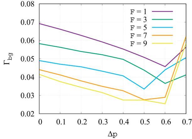
Figure 4. FoamDielExtTM target. Relative reconstruction error on the dielectric permittivity of the background ( $\Gamma_{bg}$ ) versus the number of frequencies  $F$  and the range of the Lebesgue-space exponent function  $\Delta p$ .
