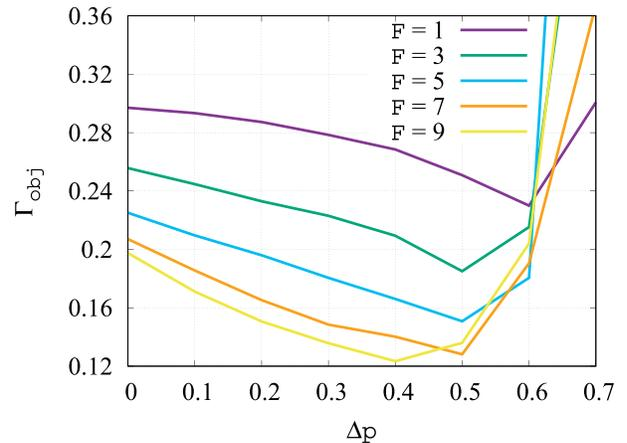
Figure 3. FoamDielExtTM target. Relative reconstruction error on the dielectric permittivity of the target ( $\Gamma_{obj}$ ) versus the number of frequencies  $F$  and the range of the Lebesgue-space exponent function  $\Delta p$ .
