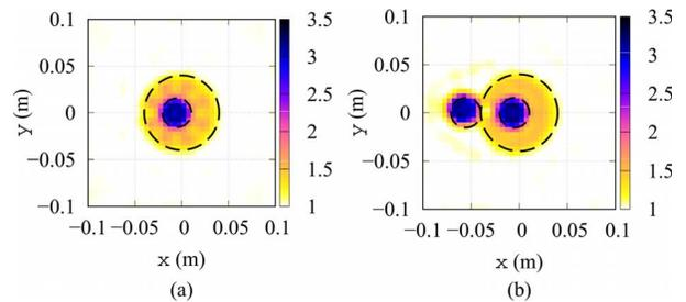
Figure 5. Reconstructed distributions of the relative dielectric permittivity of (a) the FoamDielIntTM target and (b) the FoamTwinDielTM target obtained with multifrequency processing ( $F = 9$ ,  $f = \{2, \dots, 10\}$ GHz,  $\Delta p = 0.4$ ).
