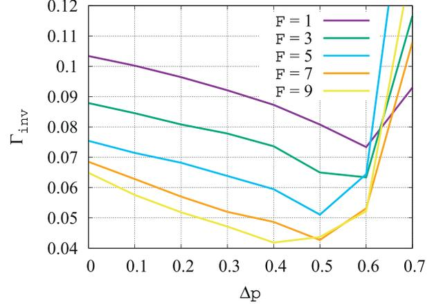
Figure 2. FoamDielExtTM target. Relative reconstruction error on the dielectric permittivity of the whole investigation domain ( $\Gamma_{inv}$ ) versus the number of frequencies  $F$  and the range of the Lebesgue-space exponent function  $\Delta p$ .
