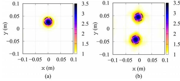
Figure 6. Reconstructed distributions of the relative dielectric permittivity of (a) the DielTM target and (b) the TwoDielTM target obtained with multifrequency processing ( $F = 7$ ,  $f = \{2, \dots, 8\}$  GHz,  $\Delta p = 0.5$ ).
