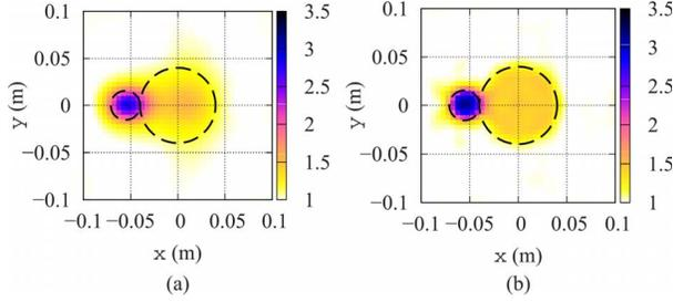
Figure 1. Reconstructed distributions of the relative dielectric permittivity of the FoamDielExtTM target obtained with (a) single-frequency processing ( $F = 1$ ,  $f = 2$  GHz,  $\Delta p = 0.6$ ) and (b) multifrequency processing ( $F = 9$ ,  $f = \{2, \dots, 10\}$  GHz,  $\Delta p = 0.4$ ).
