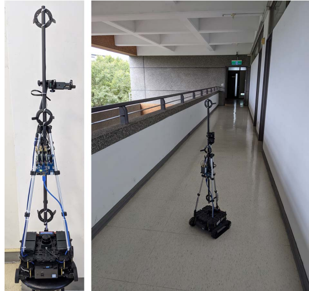
Figure 3. The site-surveying robot (left) and fingerprint gathering with SLAM in action (right).
