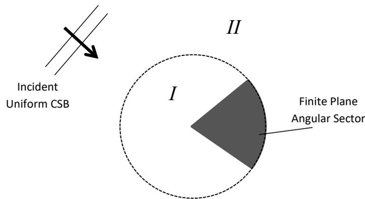
**Figure 1.** A uniform complex-source beam is illuminating a finite sector.
